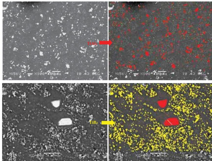
the particles including density (number/mm<sup>2</sup>), diameter and morphology.
