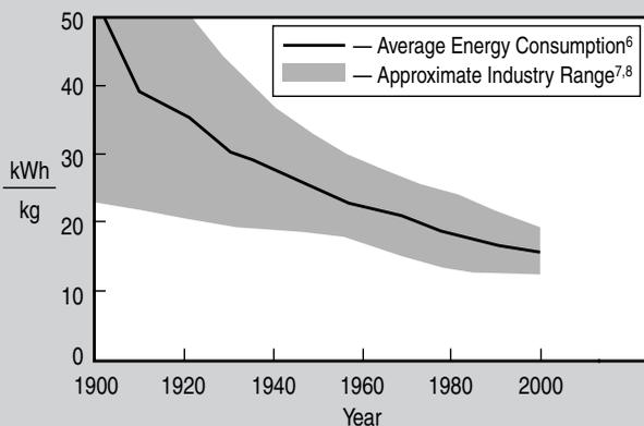
Figure 1. Historical energy efficiency improvements for aluminum smelting.
