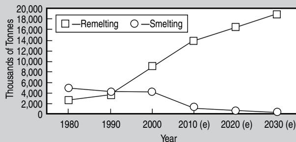
Figure 4. The U.S. trends of remelting vs. smelting.
